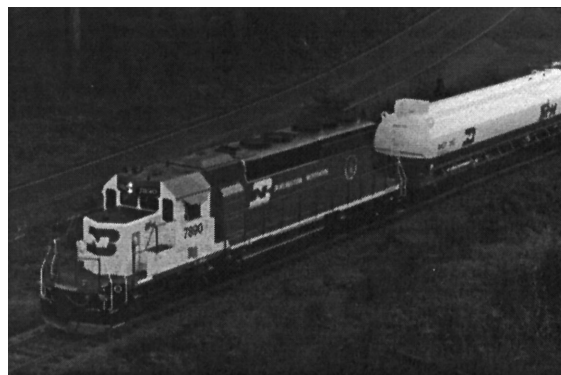
Fig. 3 BN No. 7890 natural-gas fueled locomotive
