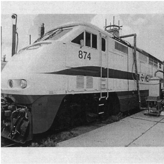
Fig. 4 Metrolink F59PHI passenger locomotive before conversion to LNG
